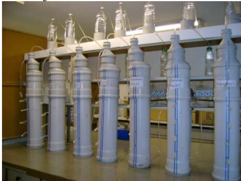
Figure 3. Pilot plant for experiment with SRB
